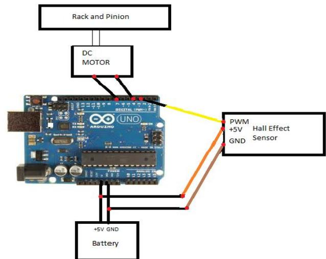
Fig. 11.Development of system according to above connections
