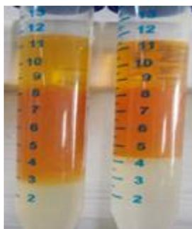
**FIGURE 5-** Lycopene forming into top hexane layer and formation of other layer with its pulp
