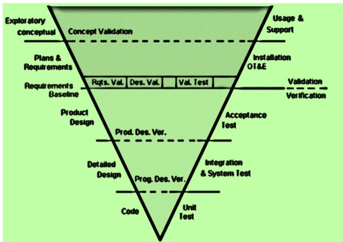
Figure 1: V-chart for the self-sterilizing System
