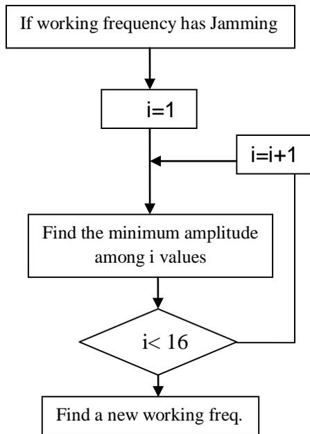
Fig.3.Jamming Analysis with fixed frequency
