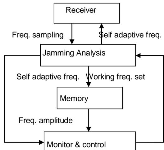
**Fig.1 Jammer module schematic chart**
