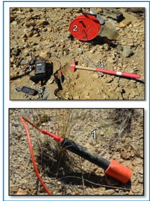
Figure 2: Equipments used for the survey ( 1 is a pair of electrode, 2 the porous pot, 3 multi-meters, 4 hammer and 5 phone)
