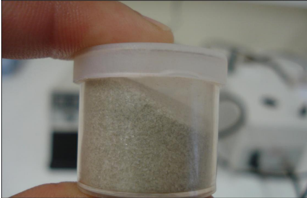
Fig. 2 – A 20ml cylindrical bottle contains Quartz and Illite sample.
