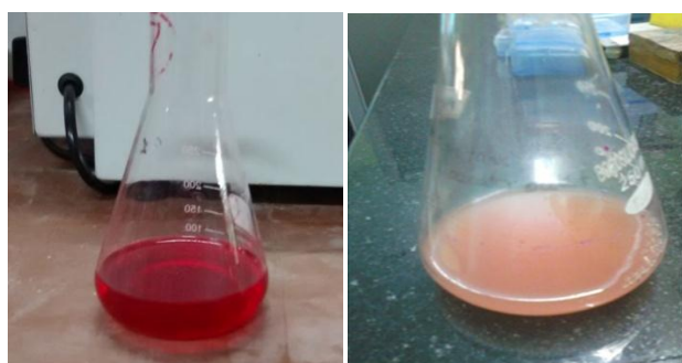
Fig 7 Synthetic dye solution at initial stage and after 3 days of incubation
