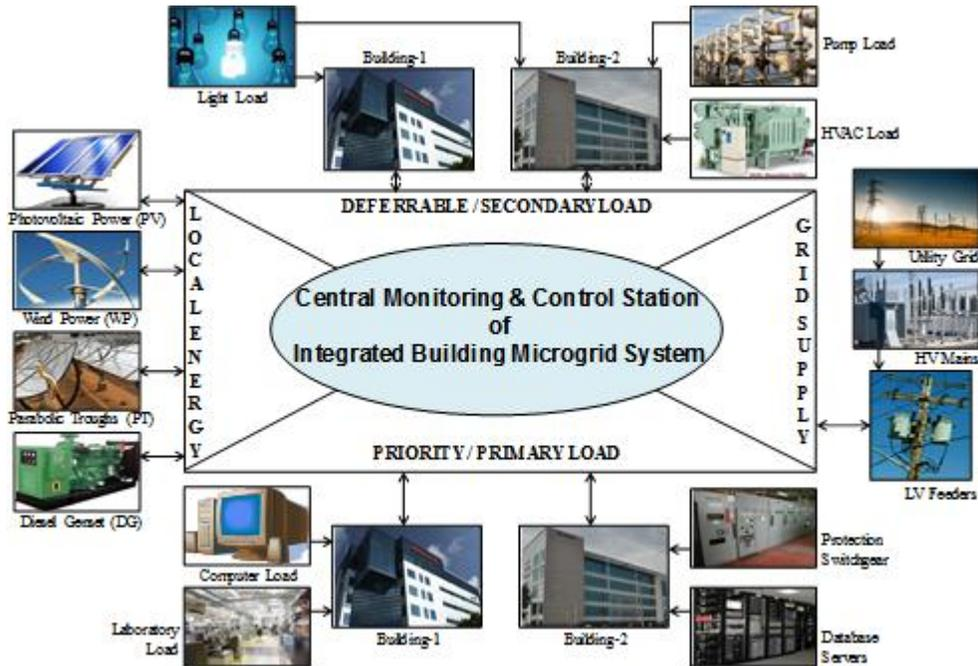
Fig. 2. Smart microgrid schematic for an industrial building.
