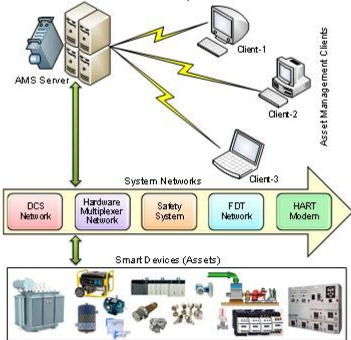
Fig. 7. AMS architecture to form a smart distribution system.
