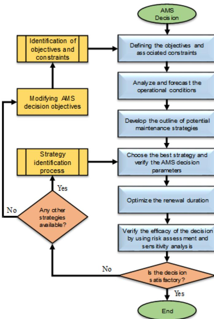
Fig. 14. AMS maintenance cycle for power plant economizer.
