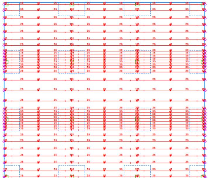
**Fig. 7. Tendons layout (x-direction).**
