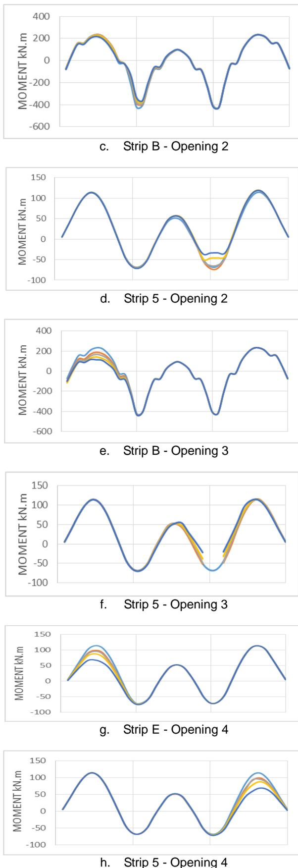
**Fig. 12.** (a- h)The bending moment diagrams for the most affected strips (7 m span)
