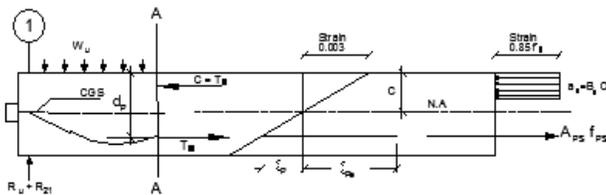
Fig. 2. Stresses and strain distribution for Post-tensioned section
