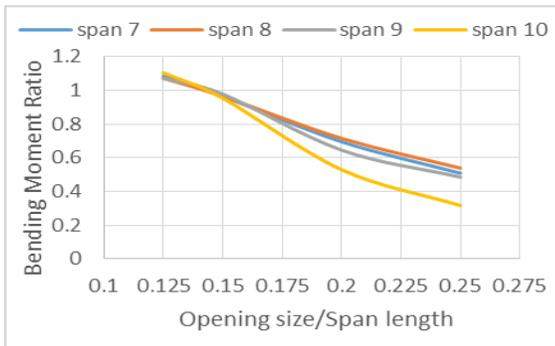
**Fig. 14.** Relation between the moment ratio for the point at strip 5 through grid B and the opening size for different span lengths for opening location 2.
