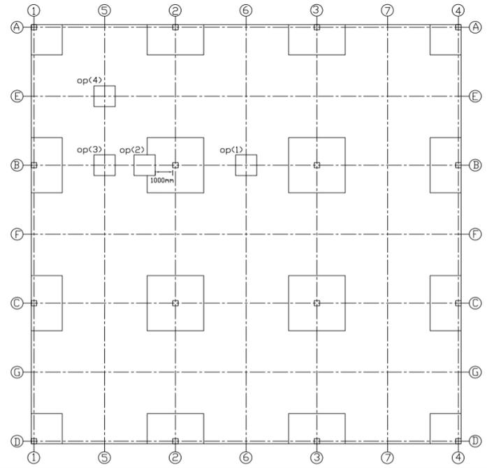
**Fig. 6. Position of openings.**
