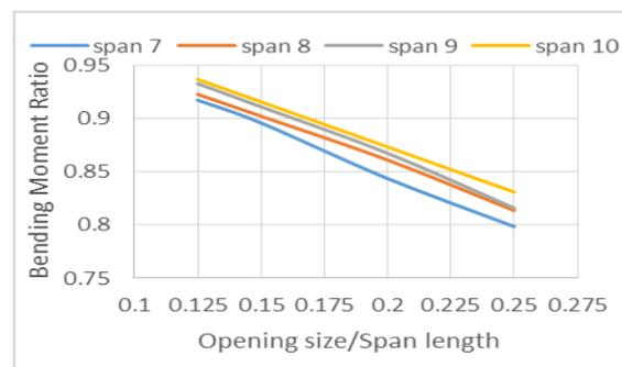
**Fig. 13.** Relation between the moment ratio for the point at strip B through grid 2 and the opening size for different span lengths for opening location 2
