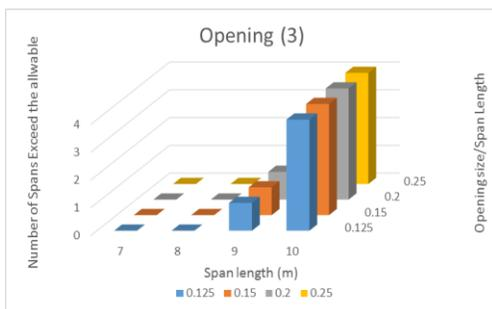
**Fig. 10. Number of spans exceeding the allowable tensile stresses for opening position 3.**
