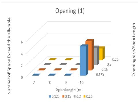
**Fig. 8. Number of spans exceeding the allowable tensile stresses for opening position 1.**
