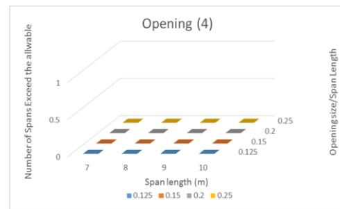
**Fig. 11. Number of spans exceeding the allowable tensile stresses for opening position 4.**
