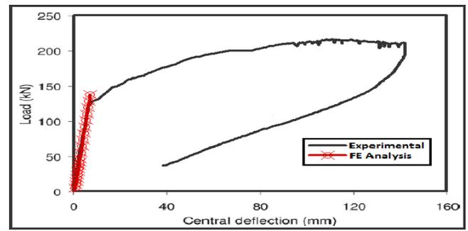
Fig. 5. Load-central deflection relationship for experimental study and our numerical model [19]
