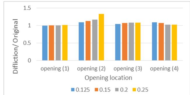
**Fig. 16.** Maximum deflection due for different opening size at different location
