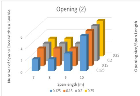
**Fig. 9. Number of spans exceeding the allowable tensile stresses for opening position 2.**
