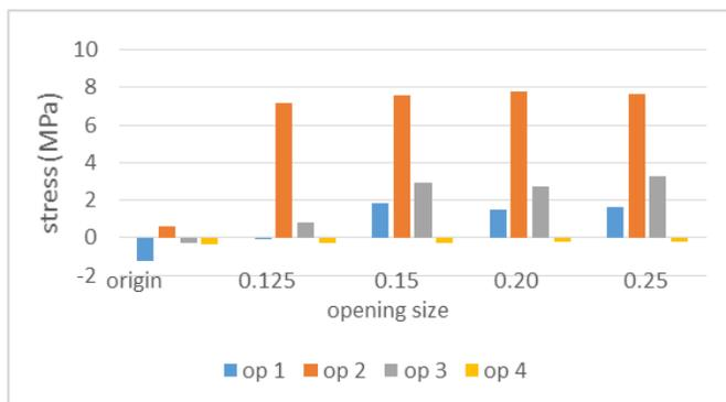
**Fig. 15.** Maximum tensile stress around openings
