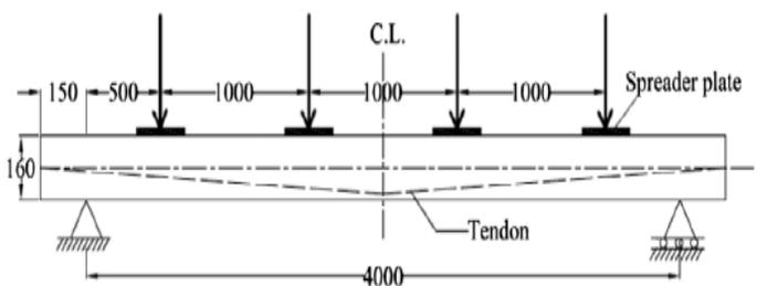
Fig. 3. Loading and general layout of slab (model TB1) [19]
