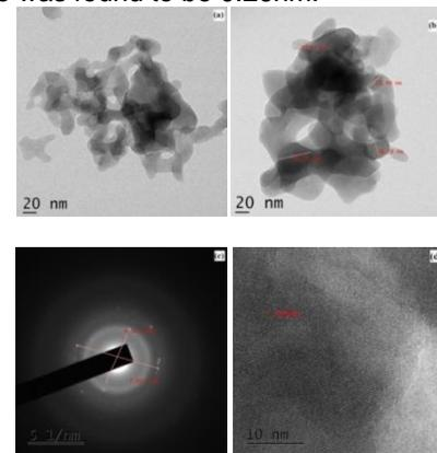
Fig. 4: TEM micrographs of  $\text{CaSiO}_3$  nanoparticles (a) TEM image (b) HR-TEM image (c) SAED Patterns (d) lattice fringes
