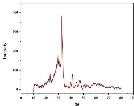
Fig. 1: XRD of synthesized calcium silicate nanoparticles
