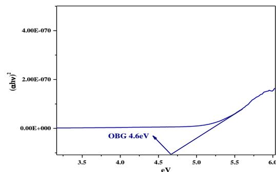
Fig. 5: Optical Band Gap of  $\text{CaSiO}_3$  nanoparticles
