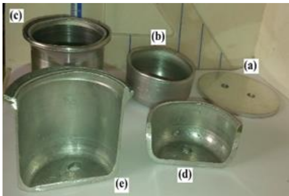
Fig. 4 Different stages of the cup production.
