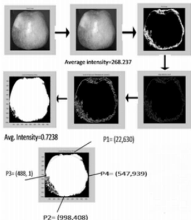
**Fig 5:** Process steps of the on-line quality assessment of test apple
