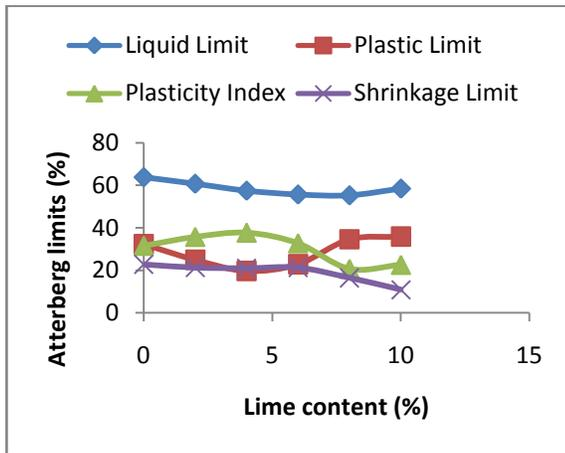
Figure 2: Atterberg Limit Test results
