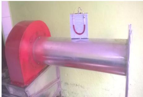
Fig. 2: Experimental performance testing of the modified centrifugal fan
