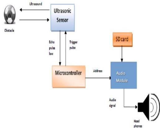
Fig 2: Distance detection using Ultrasonic sensor
