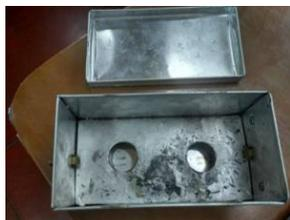
Figure 13. Solar Furnace Molder
