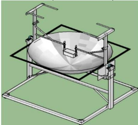
**Figure 15.** Parabolic mirror (closed container)
