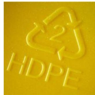
**Figure 3.** Identification Code of HDPE
