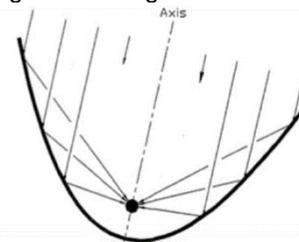
**Figure 10.** Parabolic Reflection Concept
