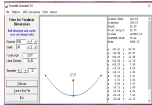
**Figure 9.** Parabolic Calculator
