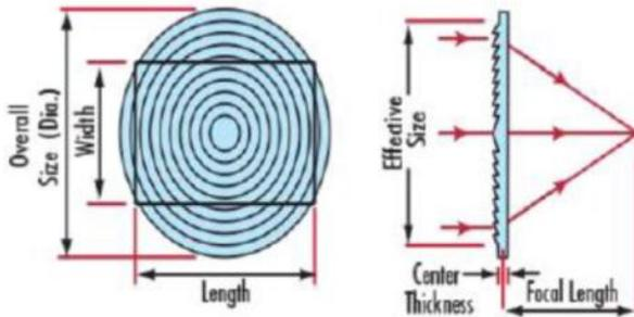
Figure 11. Concept of Fresnel Lens
