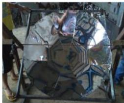
**Figure 8.** Parabolic Mirror/Reflector
