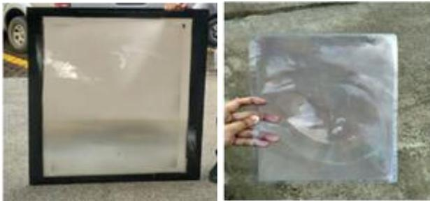
Figure 12. Linear (left) and Spot (right) Fresnel Lens.
