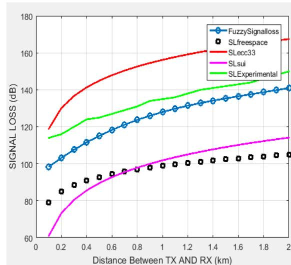
**Figure 8:** Signal loss of experimental data, the newly developed fuzzy-model and the existing models in suburban areas.
