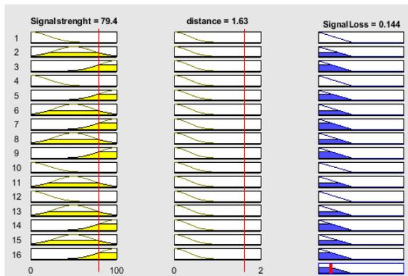
Figure2: Rule view of Fuzzy based signal loss model
