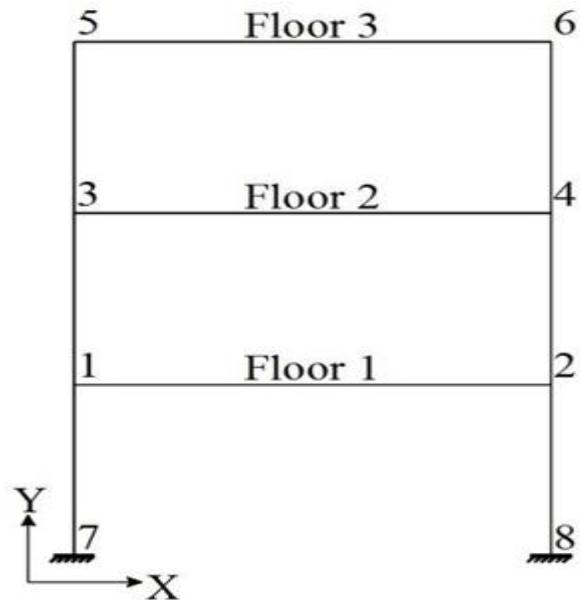
Fig. 2. A 2D frame of a single bay and three stories
