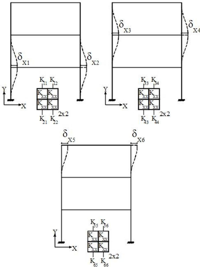
Fig. 3. Idealized stiffness matrix of the standard iteration cycle
