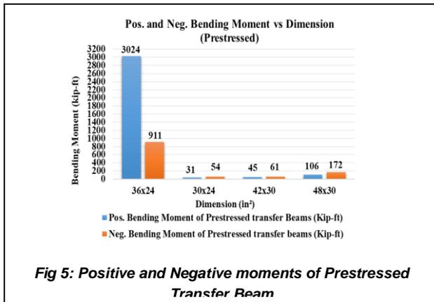
Fig 5: Positive and Negative moments of Prestressed Transfer Beam
