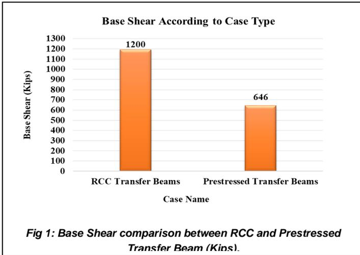
Figure 1 shows comparison between the results with the authors, it can be clearly pointed that the base shear of RCC transfer beams have about 46% higher than the prestressed transfer beams. Base shear increases with no of story increases. It shows the variation of building base shear with respect to weight of the structure.
