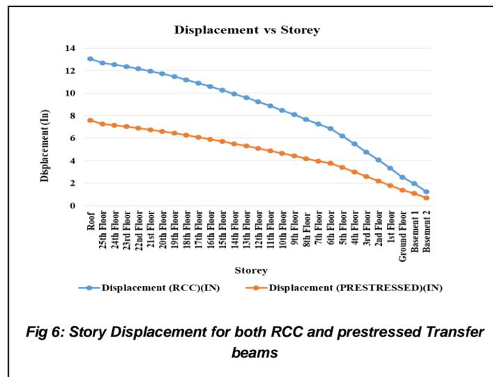
Fig 6: Story Displacement for both RCC and prestressed Transfer beams
