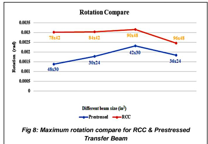
Fig 8: Maximum rotation compare for RCC & Prestressed Transfer Beam
