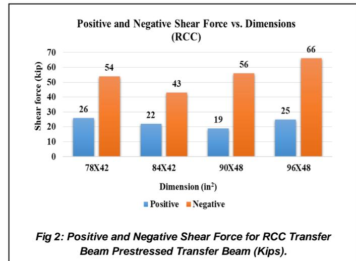
From Figure 2 it can be seen that for negative shear force for transfer beam 96x48 in<sup>2</sup> shows maximum shear and positive shear force for transfer beam 78x42 in<sup>2</sup> shows maximum shear.
