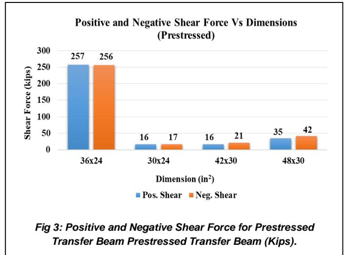
From Figure 3 it is seen that, both positive and negative shear force for transfer beam 36x24 in<sup>2</sup> shows maximum shear.
