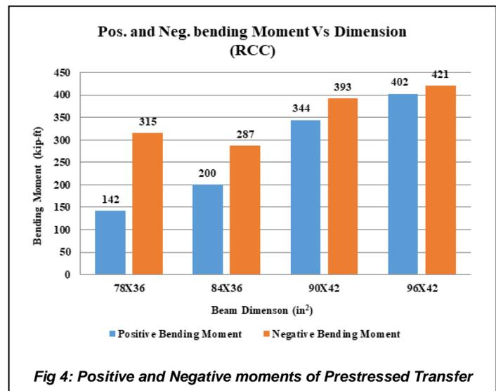
From Figure 4 it is seen that, both positive and negative bending moment for RCC transfer beam 96x42 in<sup>2</sup> shows maximum moment.
