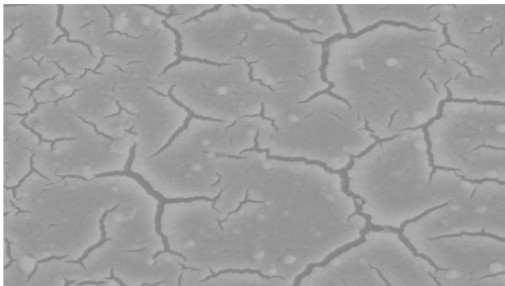
**Fig 2b:** SEM micrographs of Zinc oxide thin films using DMA as complexing agents
