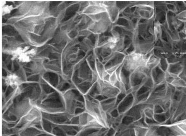
**Fig 2a:** SEM micrographs of Zinc oxide thin films without complexing agents
