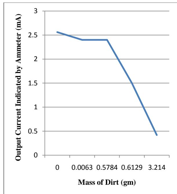
**Figure 6.3: Comparison between the dirt detecting sensor and the estimation by mass of wiped dirt for plain glass for 5 volts**
