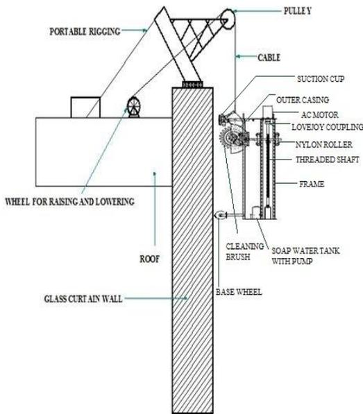
**Figure 5.1: Schematic representation showing working principle of the machine**
