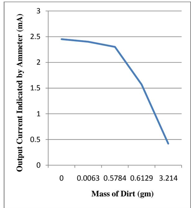
**Figure 6.2: Comparison between the dirt detecting sensor and the estimation by mass of wiped dirt for plain glass for 3 volts**
