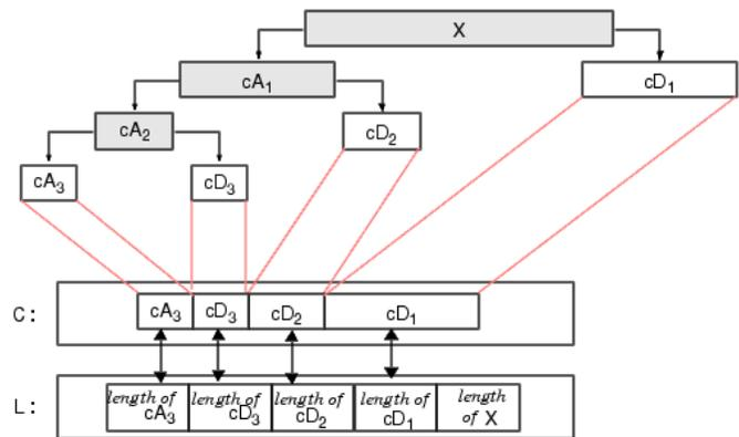
$[C,L]=wavedec(X,N,Lo\_D,Hi\_D)$  returns the decomposition structure as above, given the low- and high-pass decomposition filters you specify.
