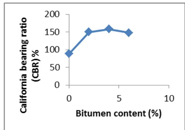
Figure 3: California bearing ratio results
