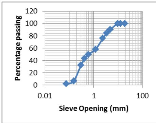
Figure 1: Particle size distribution curve of the soil sample
