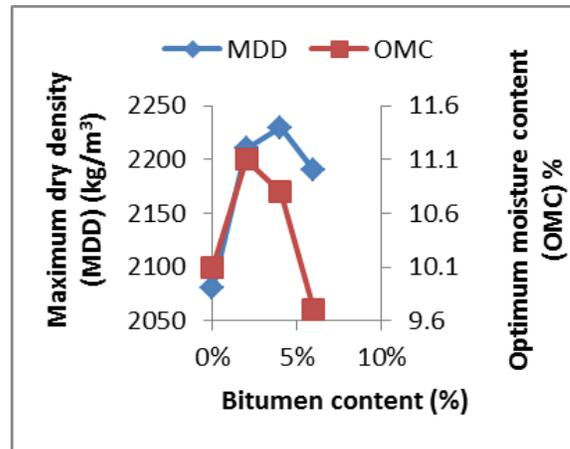
Figure 2: The relationship between maximum dry density, optimum moisture content and bitumen content
