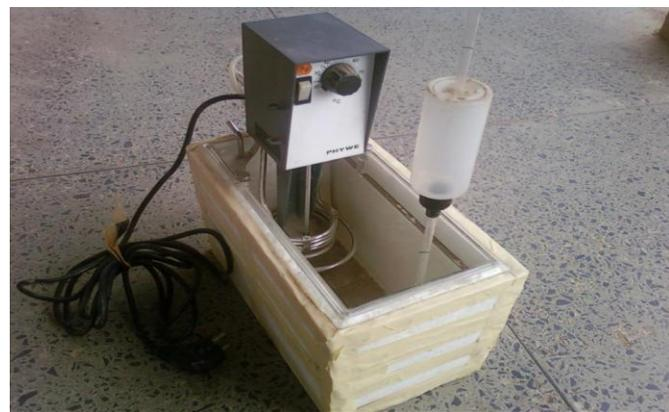
**Plate I:** Photograph of the Constructed Temperature Control Viscometer
