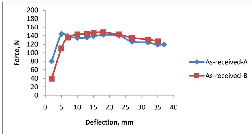
**FIG. 6: Variation of force at peak and corresponding deflection of as-received specimens**
