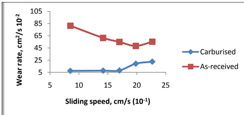
**FIG. 2: Abrasive wear rate at varying sliding speed**
