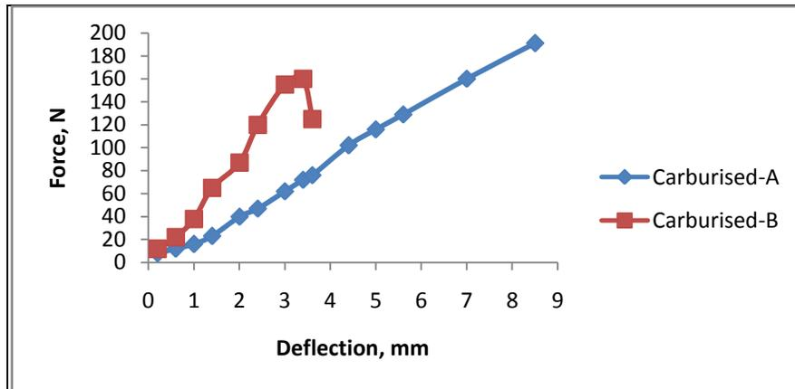
**FIG. 5: Variation of force (at peak) and corresponding deflection of carburised specimens**
