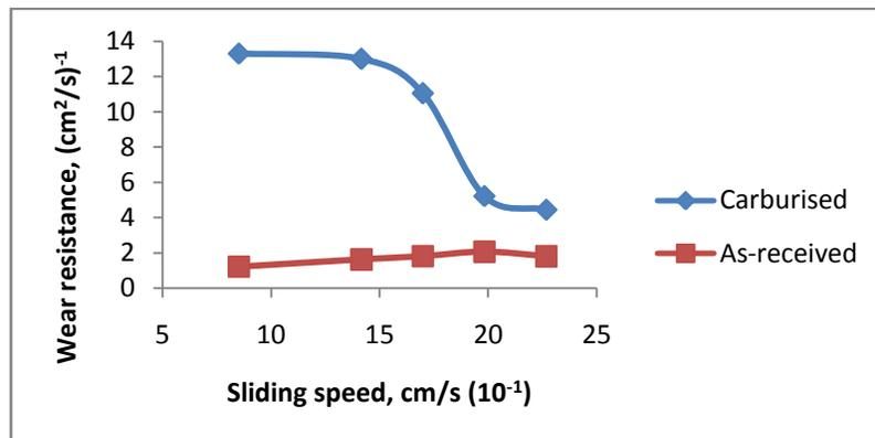
**FIG. 3: Abrasive wear resistance at varying sliding speed**
