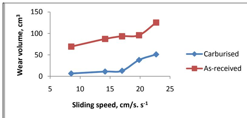
**FIG.1:** Wear volume at varying sliding speed
