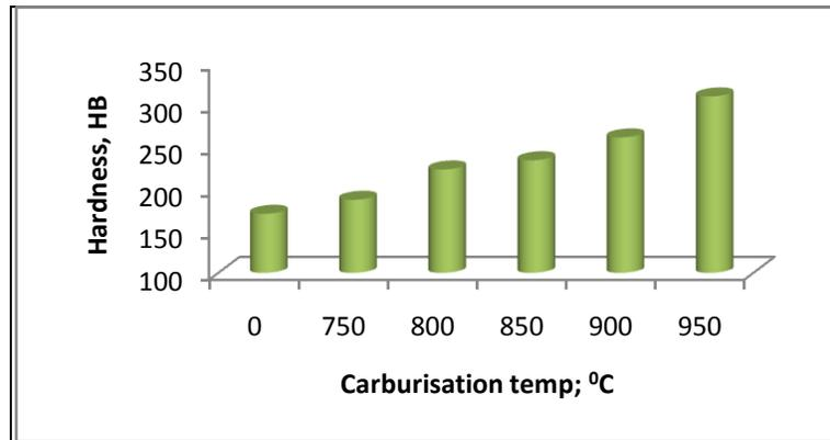
FIG. 4: Effect of carburisation temperature on hardness
