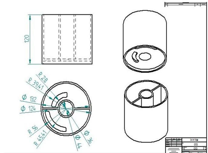
The lining also serves as a makeshift exhaust and intake manifold. The central rib separates the intake and exhaust sides and does not allow the incoming charge to mix with the exhaust gases. This ribbed design also imparts strength and stability to the assembly, minimizing vibrations and improving engine balance.
