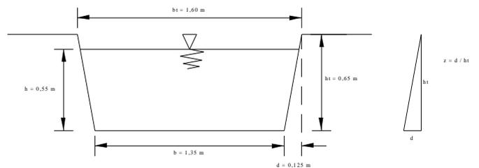
**Fig. 3.1. Diminsion of the Existing Channel**
