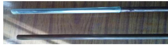
Fig. 5. COMPLETE COPPER PIPE AND (COMPOSITE PIPE)COPPER WITH SILVER (AT EVAPORATOR SECTION) HEAT PIPE
