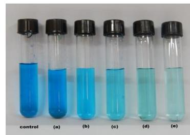
**Figure 5.** Visual observation of methylene dye degradation at different day exposure: control-without dye (a) dyesolution containing 2mg AgNPs (b) 4mg AgNPs (c) 6mg AgNPs (d) 8mg AgNPs and (e) 10mg AgNPs
