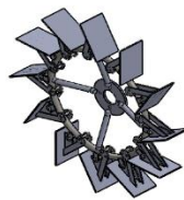
Fig. 6. Model engineering drawing of the narrow lug wheel
