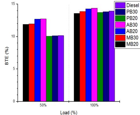
**Fig. 1** The relationship between engine load and BTE
