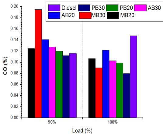
Fig. 3 The relationship between engine load and CO emission
