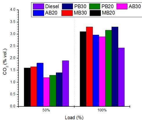
Fig. 4 The relationship between engine load and  $\text{CO}_2$  emission
