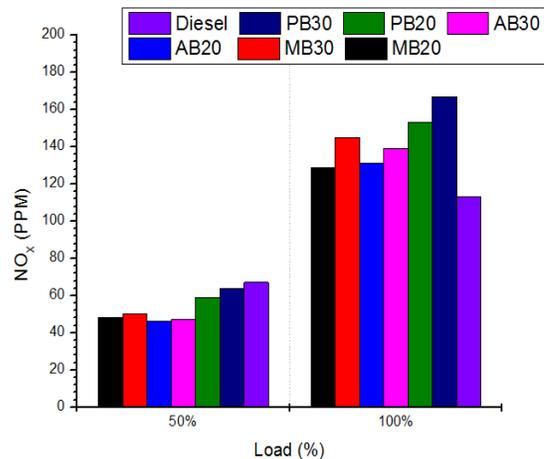
Fig. 6 The relationship between engine load and  $\text{NO}_x$
