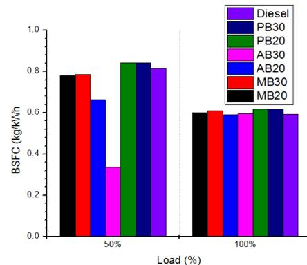
**Fig. 2** The relationship between engine load and BSFC
