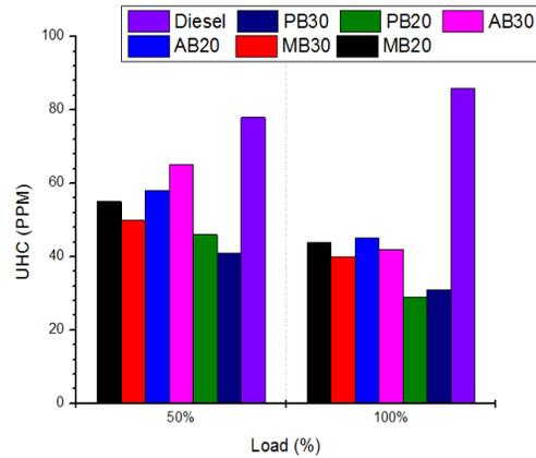
Fig. 5 The relationship between engine load and UHC
