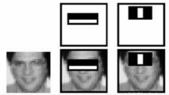
Fig. 1. Working of Haar Cascade using Edge features.
