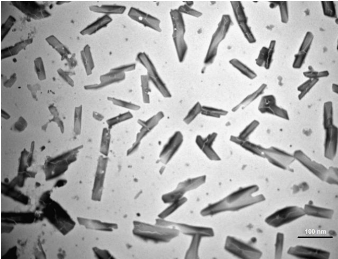
Fig.6 TEM Image of CuO Nanoparticles
