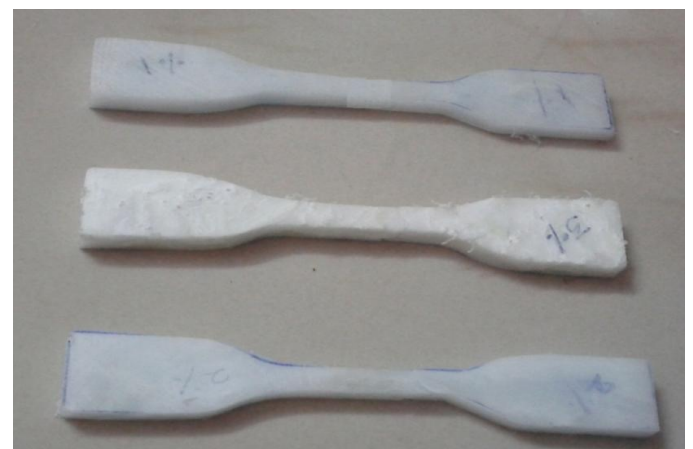
Fig.2. Specimens for Tensile Test
