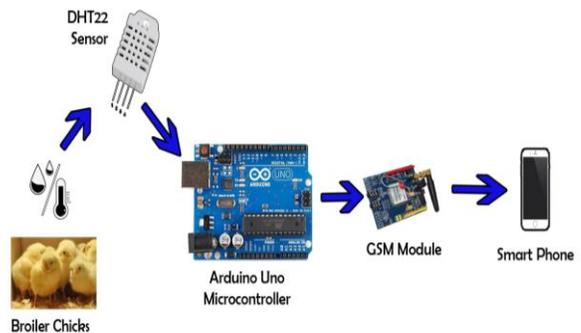
**Fig. 4.** System Architecture Framework.
