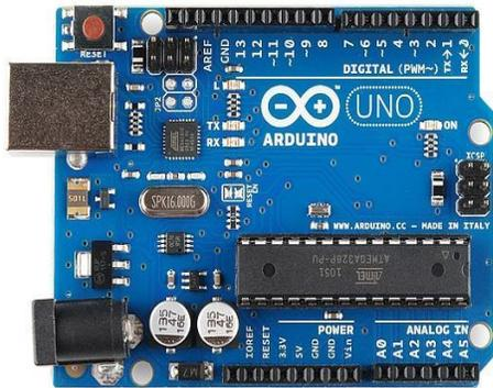
**Fig. 1.** Arduino Uno Microcontroller. The Arduino is the main controller of the developed prototype. All the data detected from the DHT22 sensor is process by the microcontroller.
