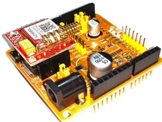
**Fig. 3.** GSM Module. The GSM Module is connected to the Arduino Microcontroller. Through the GSM Module, the information about the temperature level and humidity level is sent to the mobile phone of the poultry farmer through a text message.
