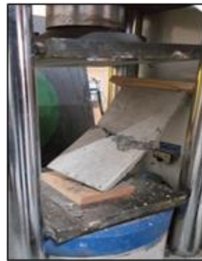
Figure 4.2 Individual ferrocement panel and LGS channel
