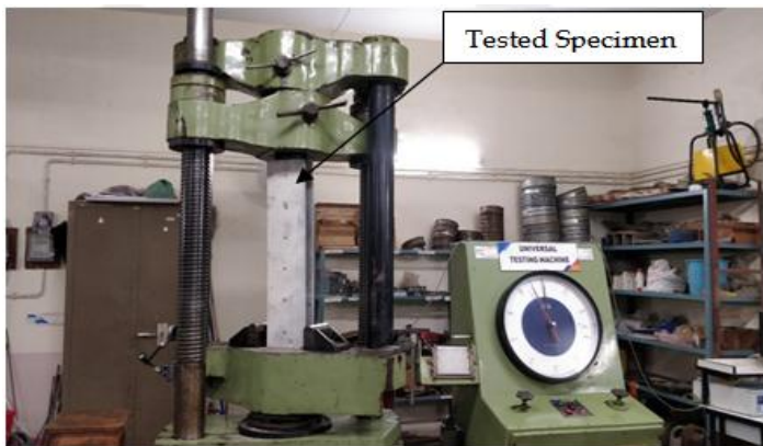
Figure 4.3 Arrangement of compression specimen on UTM
