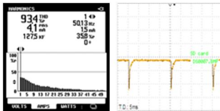
Fig. 1. Total harmonic distortion and distorted current waveform of tested unit 1
