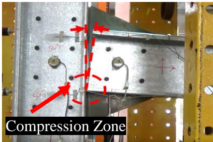
Fig. 10. Deformation of HG-BGJ-7 specimen
