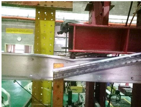
Fig. 15. The web beam was buckling
