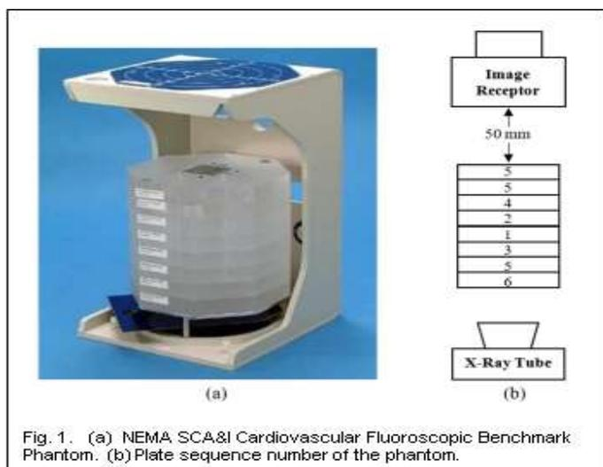
Fig. 1. (a) NEMA SCA&I Cardiovascular Fluoroscopic Benchmark Phantom. (b) Plate sequence number of the phantom.
