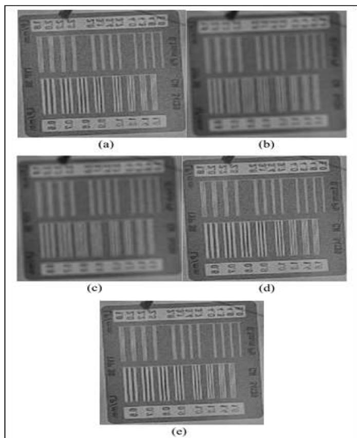
**Fig. 3.** Images of fluoroscopy NEMA SCA&I Cardiovascular Fluoroscopic Benchmark Phantom; (a) Original image; (b) Image after MF filtering; (c) Image after AMF filtering; (d) Image after BF filtering; (e) Image after SMF filtering.
