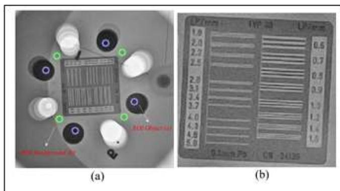
Fig. 2. (a) Determination of ROI for measuring SNR and CNR, and (b) Line pairs object for assessment of the spatial resolution of the image within the NEMA SCA&I Cardiovascular Fluoroscopic Benchmark Phantom.
