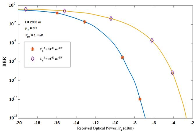
**Fig. 5** BER vs. Received optical power over different refractive index variations for  $L = 2$  km.
