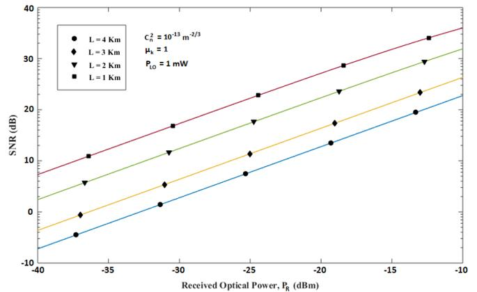
Fig. 2 SNR vs. Received optical power
