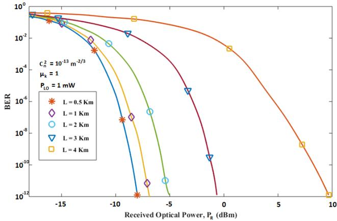
**Fig. 3** BER vs. Received optical power for  $\mu_k = 1$
