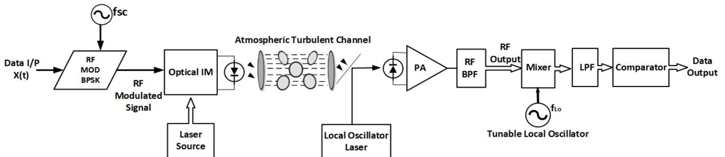
Fig. 1 Simplified Diagram of Coherent FSO link with single RF sub-carrier modulation under strong turbulent channel
